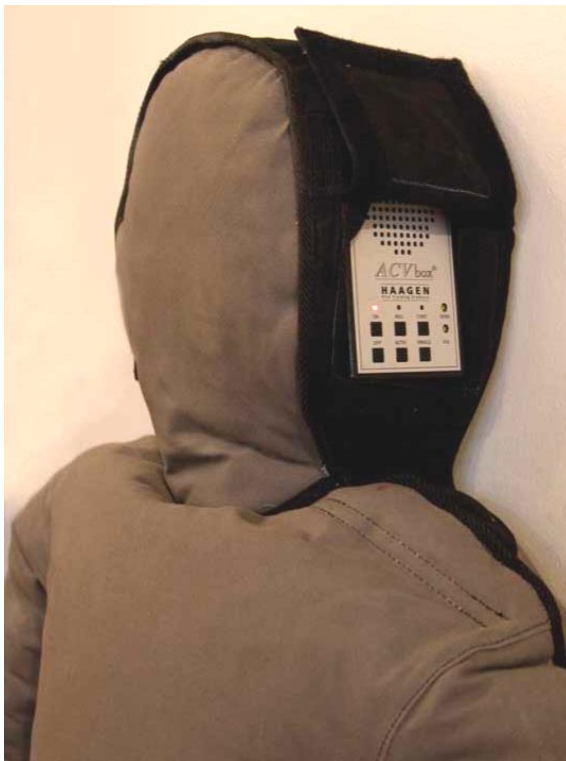
Figure 6: ACV Box inside the Head of the 'SmartDummy™ Thermal'
